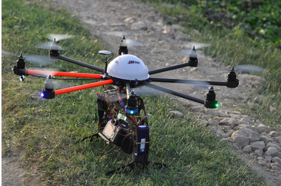
Figure 2.10: Octocopter with GPS and Canon 5D (50 mm lens) mounted
