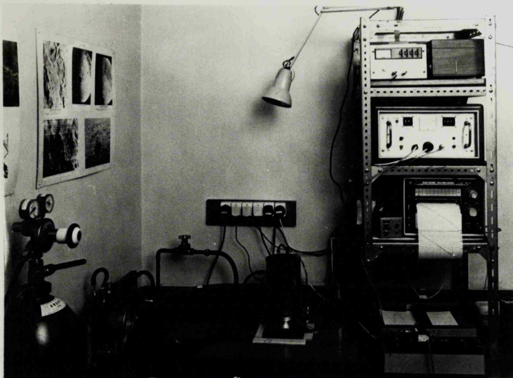
Figure II.1a Photograph of the assembled thermoluminescence apparatus. The photomultiplier tube housing is in the centre resting on the specimen chamber. This is evacuated and filled with an inert gas via the vacuum line on the left. A Dewar flask containing the cold-junctions for the thermocouples stands at the back of the rack which holds the HT unit (top), the control unit, the amplifier and a chart recorder to check the heating rate. At the base of this is the XY recorder and below the bench is a constant-voltage transformer for the control unit
