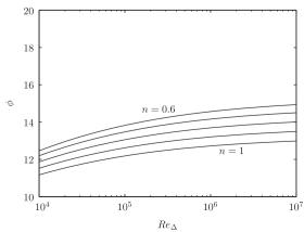
Fig. 3. Plots of the asymptotic neutral wavenumber  $k_{\Delta}$  and wave angle  $\phi$  predictions for n = 1, 0.9, 0.8, 0.7 and 0.6 using two terms of the asymptotic results.
