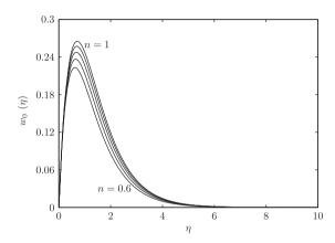
**Fig. 2.** The inviscid motion eigenfunction  $w_0(\eta)$  for n = 1, 0.9, 0.8, 0.7, 0.6.
