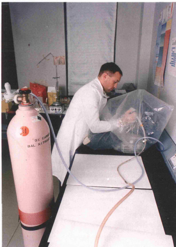
Figure 4.2: Photograph Showing the ATMOSBAG filled with 95% Nitrogen/5% Carbon Dioxide for Handling of Deoxygenated Culture Medium in a Deoxygenated Environment.
