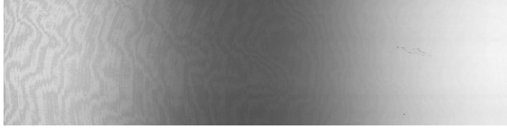
Figure 2.5: Example flat-field image taken with the Gemini South telescope.
