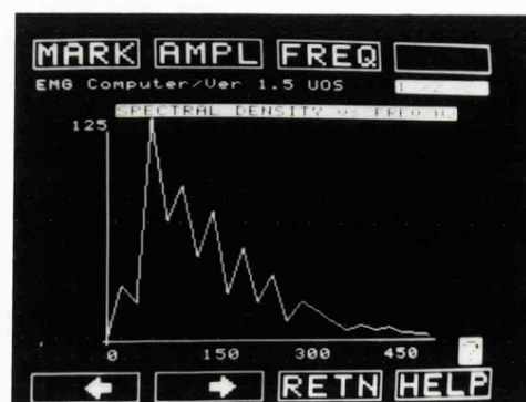
Fig.[3.12] Some display formats available under 'MUSCLE', the EMG Turning Points Spectral Analysis Application for the SPC.
