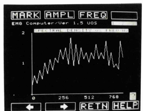
Fig.[3.12] Some display formats available under 'MUSCLE', the EMG Turning Points Spectral Analysis Application for the SPC.
