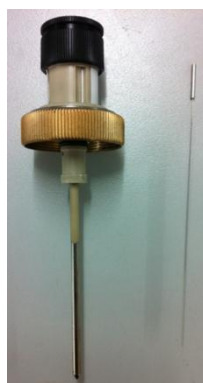
Figure 4.3 Sample inlet probe purchased from AB Sciex UK Limited, Cheshire, UK
