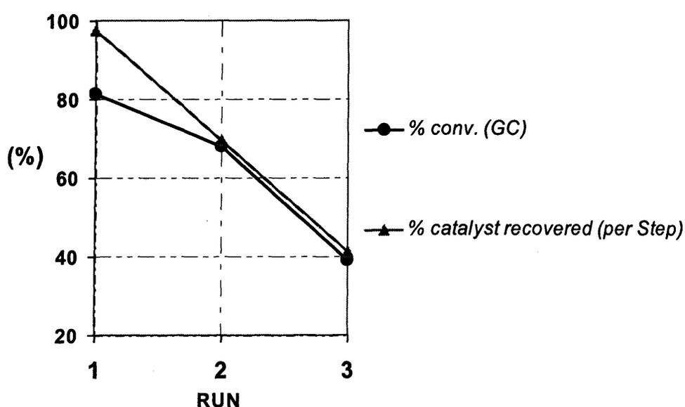
**Figure 5.12.** Recycling of dibenzo-crown ether [4.27] using thermomorphic catalysis.
