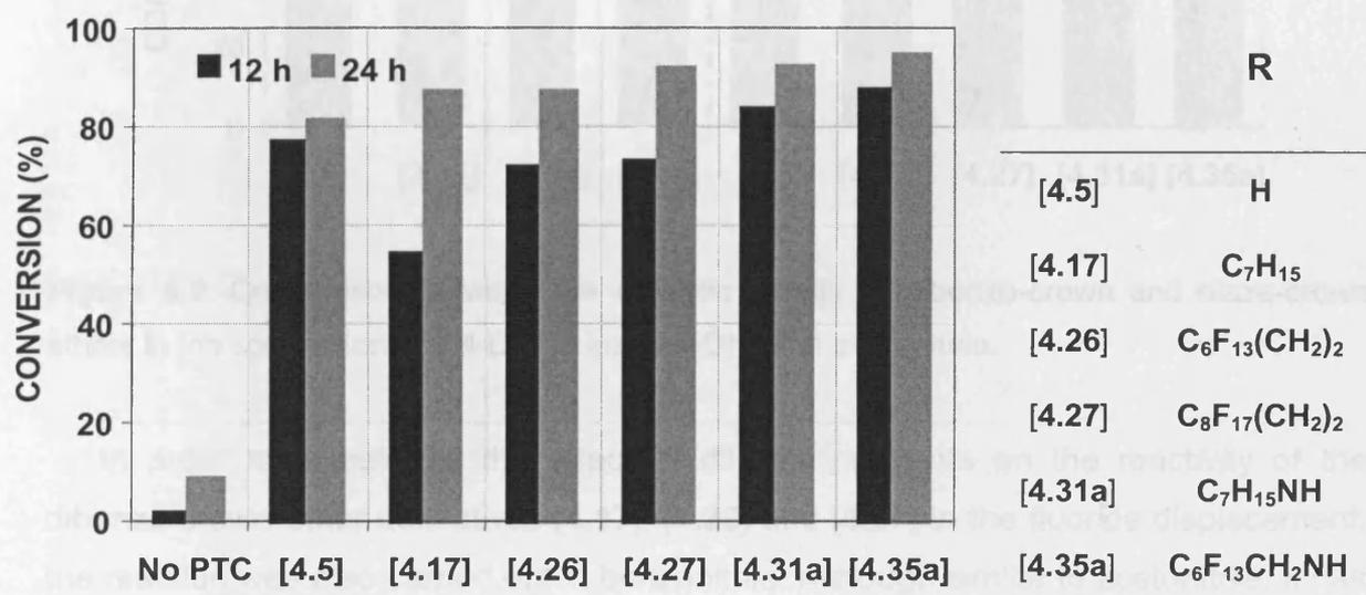
**Figure 5.8.** Phase transfer catalytic activity of dibenzo-crown ethers in the conversion of 2,4-DNCB into 2,4-DNFB in acetonitrile under solid-liquid conditions.
