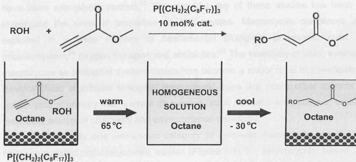
**Scheme 1.8.** Addition of alcohols to methyl propiolate catalysed by a thermomorphic fluororous phosphine.
