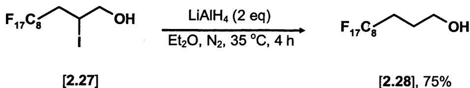
**Scheme 2.8.** Synthesis of the partially fluorinated alcohol 1*H*,1*H*,2*H*,2*H*,3*H*,3*H*-perfluoro-*n*-undecanol, [2.28].
