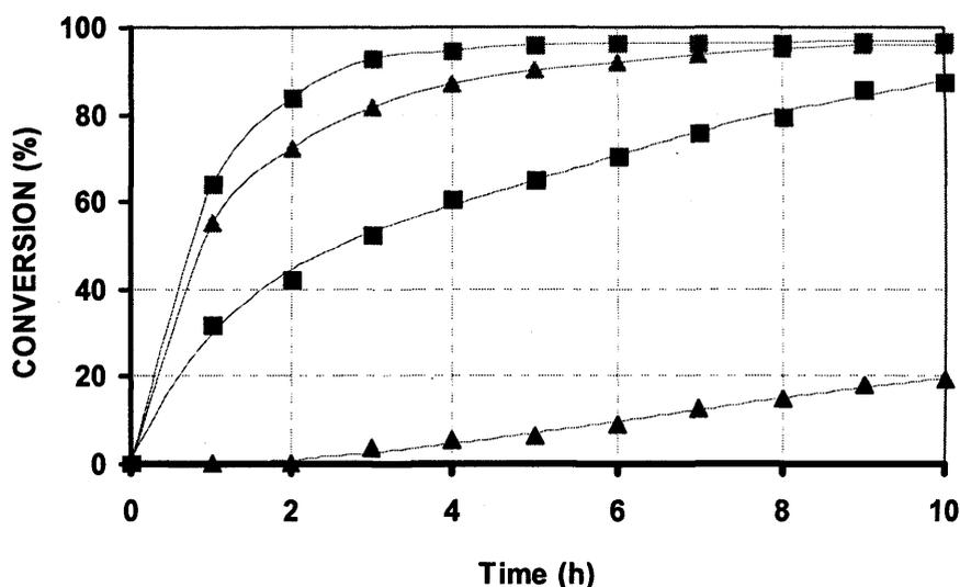
**Figure 3.4.** Phase transfer catalytic activity of diaza-crown ethers [2.6] and [2.36] in the conversion of  $n$ -C<sub>8</sub>H<sub>17</sub>Br into  $n$ -C<sub>8</sub>H<sub>17</sub>I in benzotrifluoride and toluene under solid-liquid conditions.
