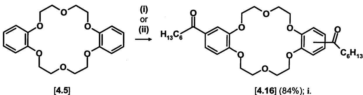
(i)  $\text{C}_6\text{H}_{13}\text{CO}_2\text{H}$  [4.14], PPA, 1 h, 90 °C.
