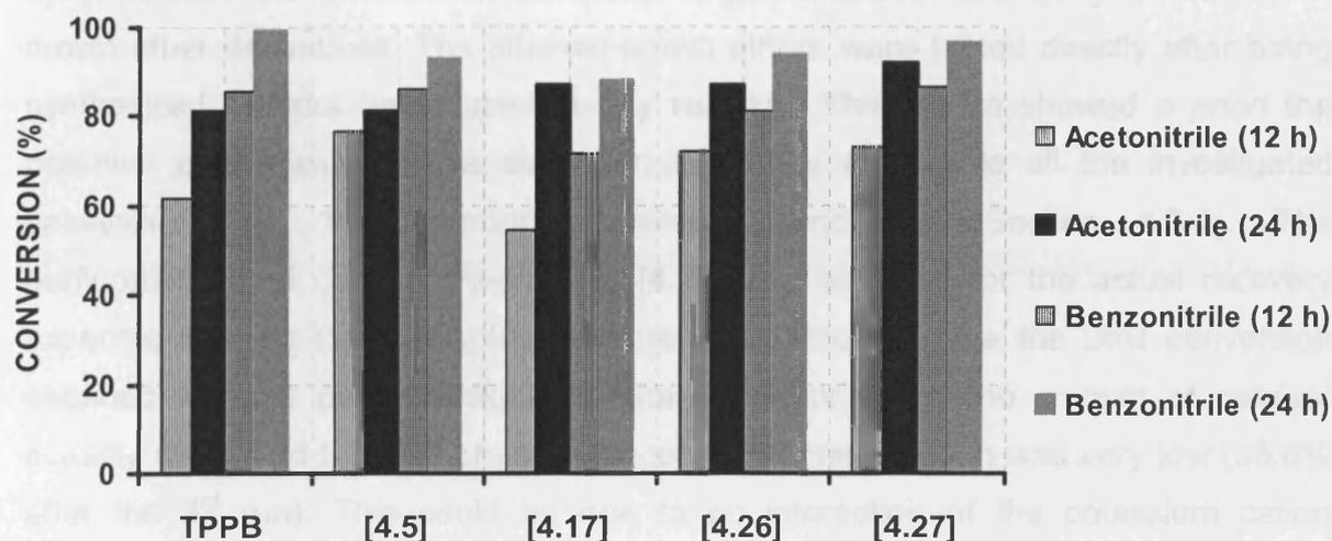
**Figure 5.10.** Comparison between the catalytic activities of dibenzo-crown ethers and TPPB in the conversion of 2,4-DNCB into 2,4-DNFB in acetonitrile and benzonitrile after 12 h and 24 h.
