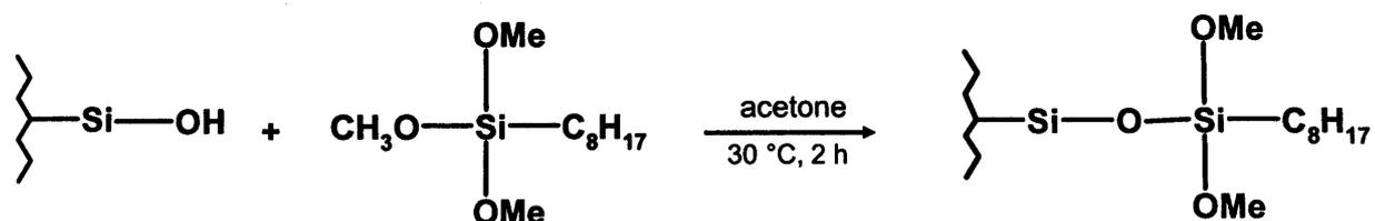
**Scheme 1.4.** Synthesis of Reverse Phase Silica.
