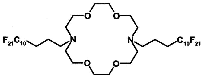
A solution of 4,13-diaza-18-crown-6 (0.20 g, 0.8 mmol), cesium carbonate (0.50 g, 1.5 mmol) and 1*H*,1*H*,2*H*,2*H*,3*H*,3*H*-perfluoro-*n*-tridecyl iodide (1.10 g, 1.6 mmol) in acetonitrile (30 mL) was heated at 85
