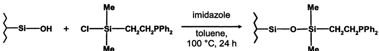
**Scheme 1.3.** Synthesis of Silica Solid Support.
