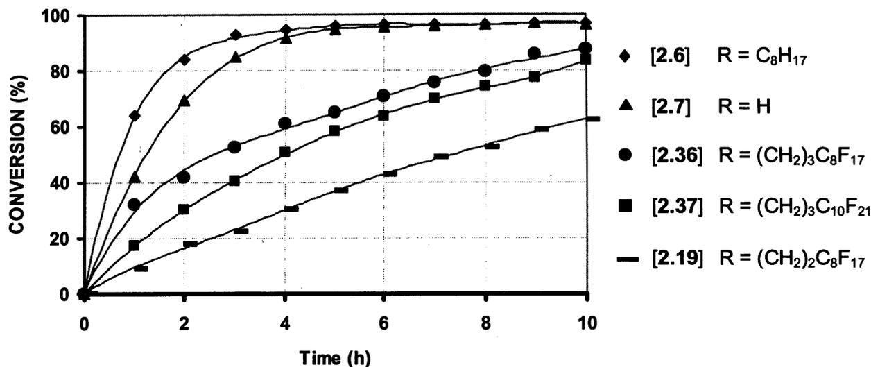
**Figure 3.3.** Phase transfer catalytic activity of diaza-crown ethers in the conversion of *n*-C<sub>8</sub>H<sub>17</sub>Br into *n*-C<sub>8</sub>H<sub>17</sub>I in benzotrifluoride under solid-liquid conditions.
