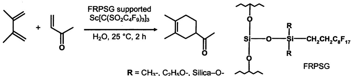
**Scheme 1.6.** Diels-Alder reaction using FRPSG supported catalyst.
