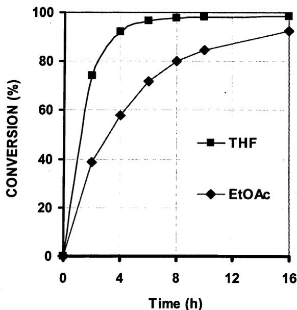
**Figure 5.11.** Catalytic activities of dibenzo-crown ether [4.26] supported on FRPSG in THF and EtOAc.
