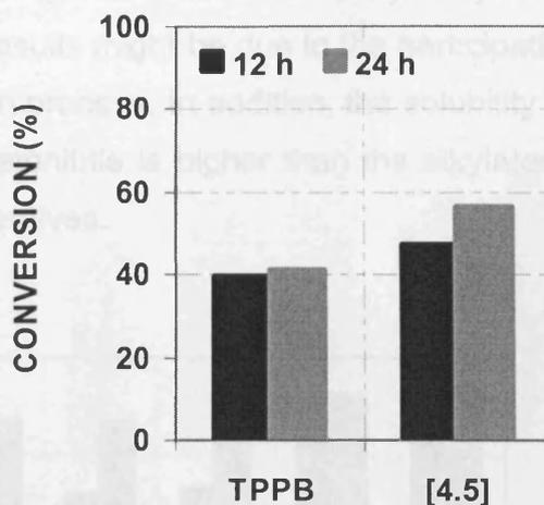
**Figure 5.7.** Catalytic activities of 5 mol % of phase transfer catalysts TPPB and dibenzo-crown ether [4.5] in the conversion of 2,4-DNCB into 2,4-DNFB in acetonitrile with 3 eq. of KF after 12 h and 24 h.
