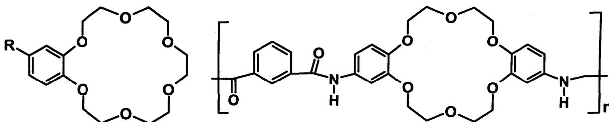
**Figure 1.9.** Polymer-supported crown ethers.
