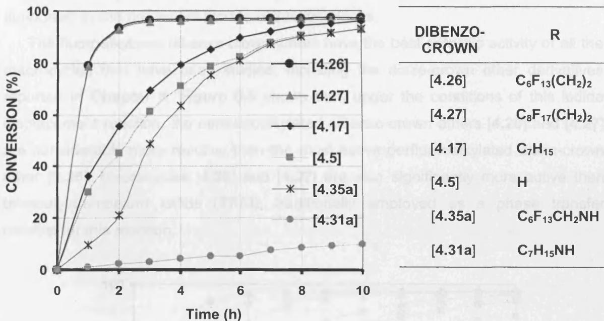
**Figure 5.4.** Phase transfer catalytic activity of dibenzo-crown ethers in the conversion of  $n$ -C<sub>8</sub>H<sub>17</sub>Br into  $n$ -C<sub>8</sub>H<sub>17</sub>I in benzotrifluoride under solid-liquid conditions.
