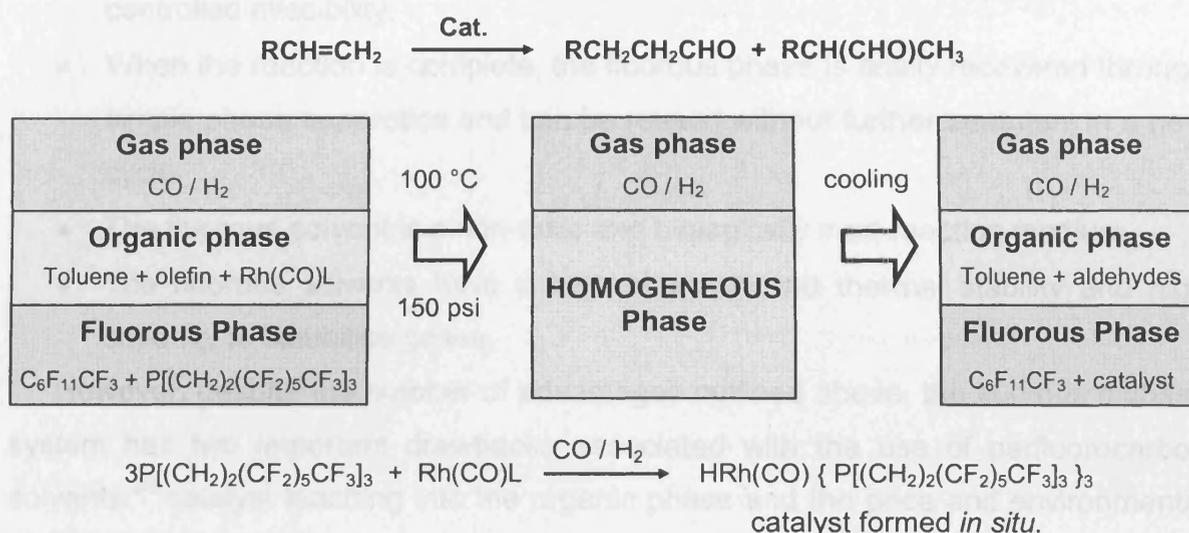
**Scheme 1.2.** Hydroformylation of Olefins in the Fluorous Biphasic System.
