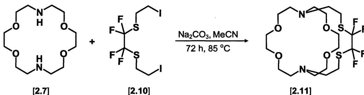
**Scheme 2.5.** Synthesis of the first fluorinated cryptand capable of forming stable complexes with metal cations.
