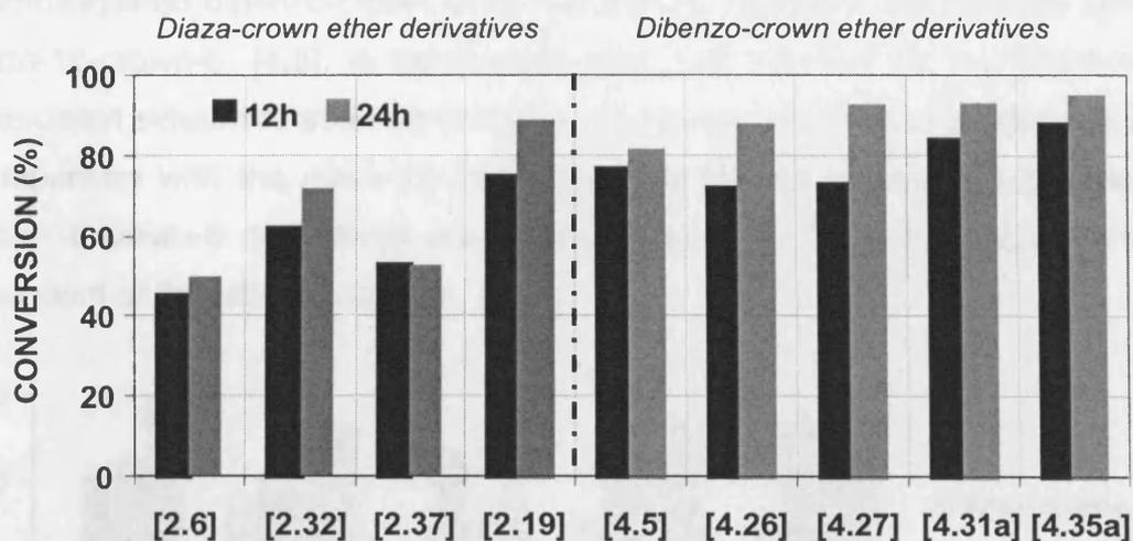
**Figure 5.9.** Comparison between the catalytic activity of dibenzo-crown and diaza-crown ethers in the conversion of 2,4-DNCB into 2,4-DNFB in acetonitrile.
