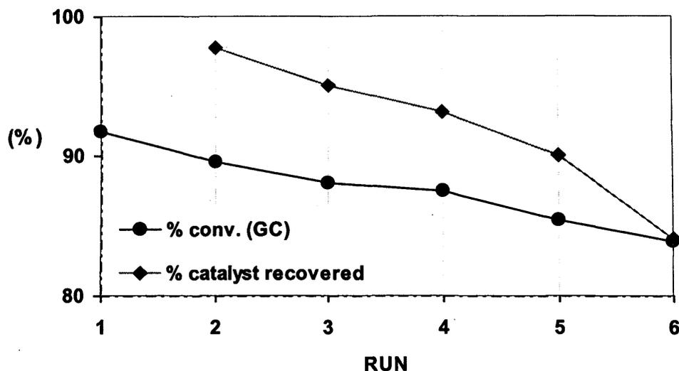
**Figure 3.5.** Separation and recovery of fluorinated diaza-crown ether [2.36] by SPE.
