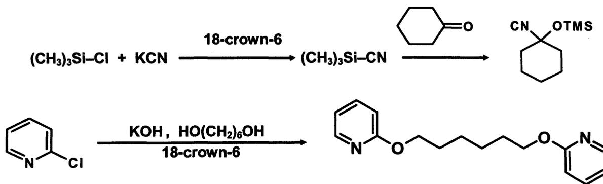
**Scheme 1.11.** Crown Ethers as Phase Transfer Catalysts.
