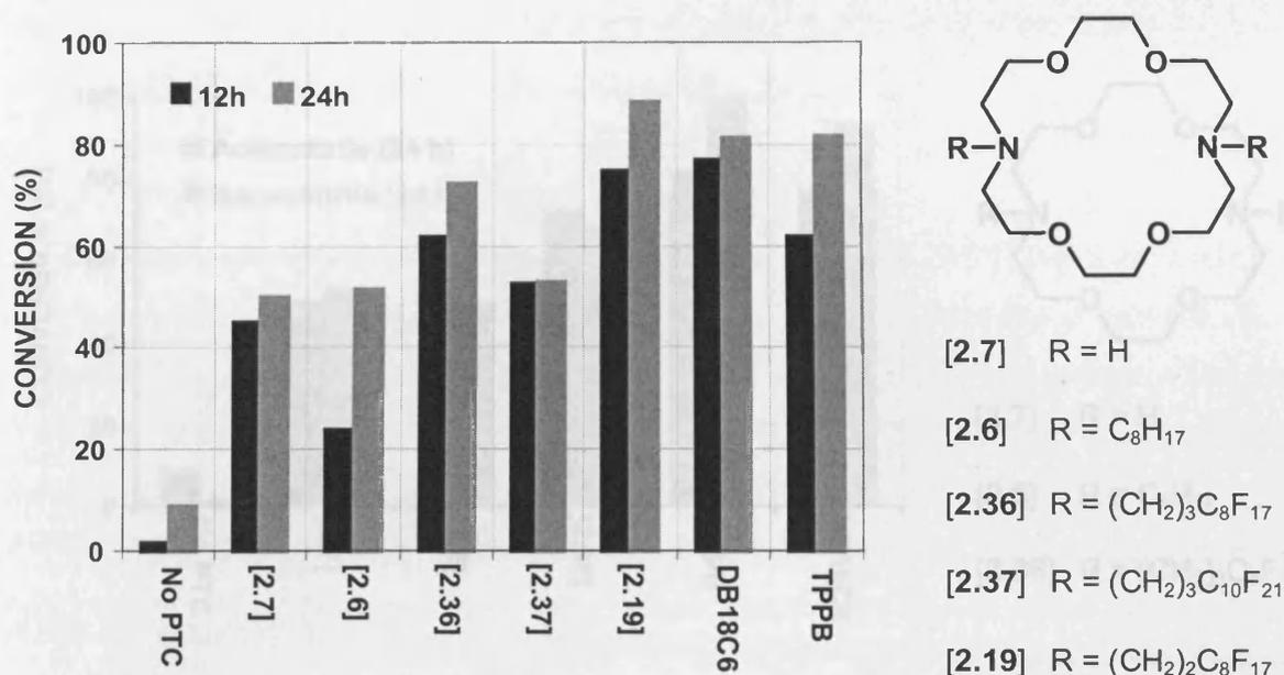
Figure 3.7 Phase transfer catalytic activity of diaza-crown ethers in the fluorination of 2,4-dinitrochlorobenzene in acetonitrile under solid-liquid conditions.
