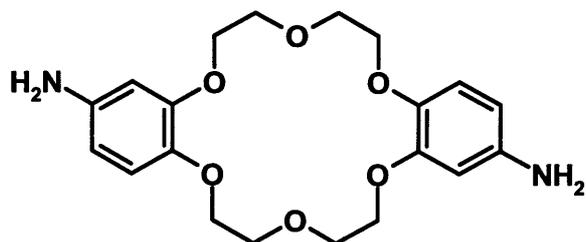
*Trans*-di(nitrobenzo)-18-crown-6 (2.60 g, 6.0 mmol) was dissolved in hot *N,N*-dimethylformamide (70 mL). 10% Pd/C (0.60 g) was added and the reactor was placed in a pressurized hydrogenation apparatus. The reactor was charged with
