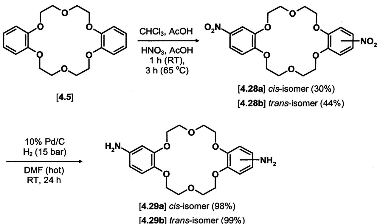
**Scheme 4.7.** Synthesis of *cis*- and *trans*-di(aminobenzo)-18-crown-6.
