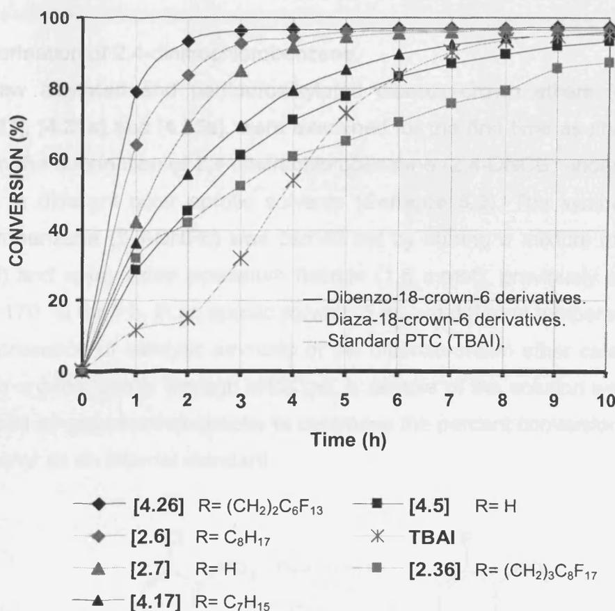
**Figure 5.5.** Comparison between the catalytic activity of diaza-crown and dibenzo-crown ether derivatives in the conversion of  $n\text{-C}_8\text{H}_{17}\text{Br}$  into  $n\text{-C}_8\text{H}_{17}\text{I}$  under solid-liquid conditions.
