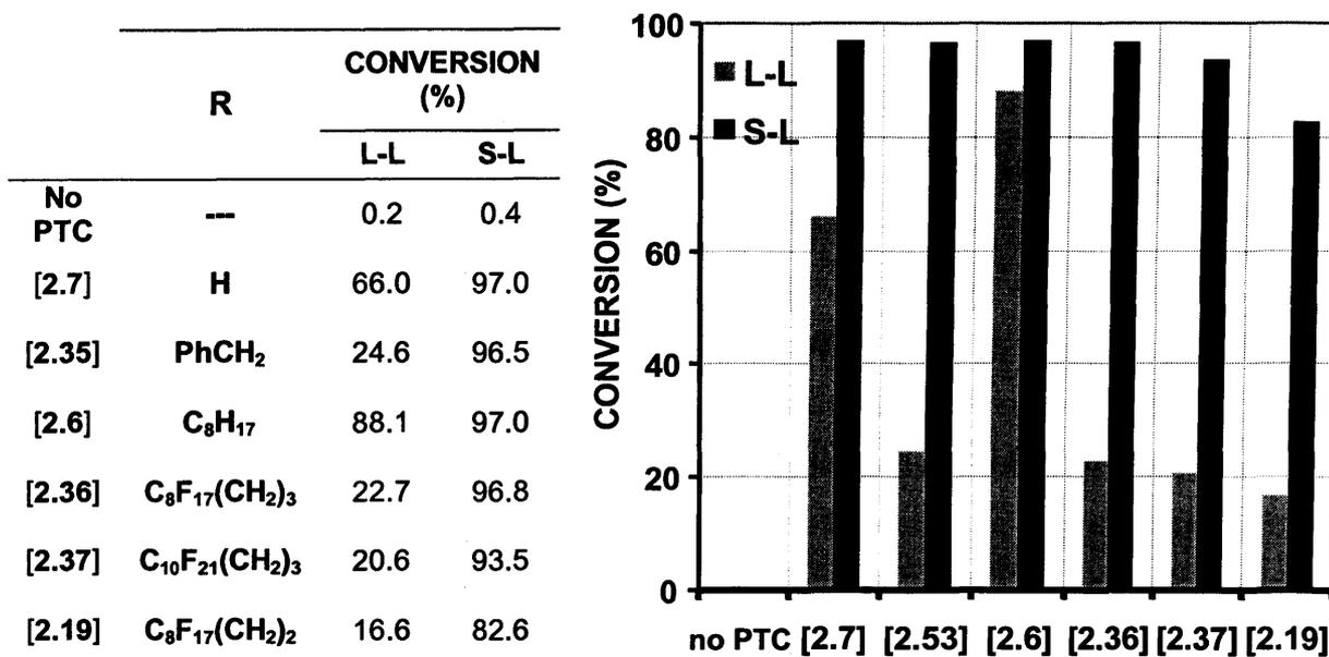
**Figure 3.2.** Phase transfer catalytic activity of diaza-crown ethers in the conversion of  $n$ -C<sub>8</sub>H<sub>17</sub>Br into  $n$ -C<sub>8</sub>H<sub>17</sub>I in benzotrifluoride under liquid-liquid and solid-liquid conditions.
