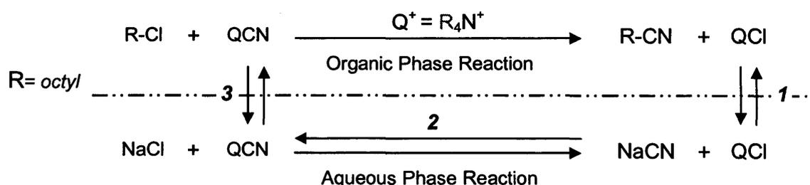
**Scheme 1.12.** Schematic representation of phase transfer-catalysed cyanide displacement in 1-chlorooctane.
