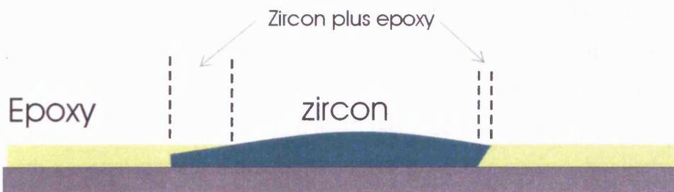
Fig. 9.16. Indication of the importance of truly flat zircon surface.
