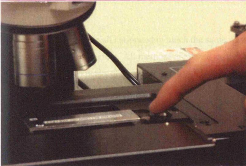
Fig. 3.12. Loading a slide on the mapping stage beneath the objective.
