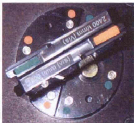
Fig. 3.7. Software-controlled double-sided grating.
