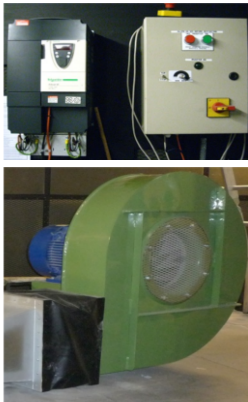
Figure 3.10: The blower fan (below) and its frequency controller (above)
