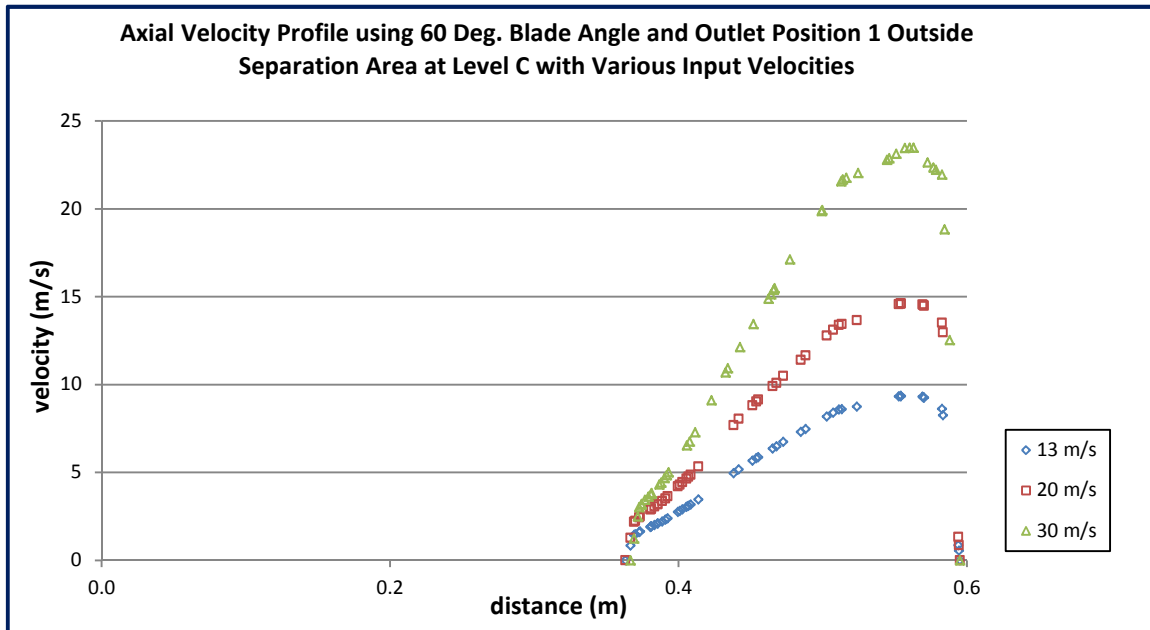
Axial velocity profile outside separation area at Level C for various input velocities (60 degrees vane angle)
