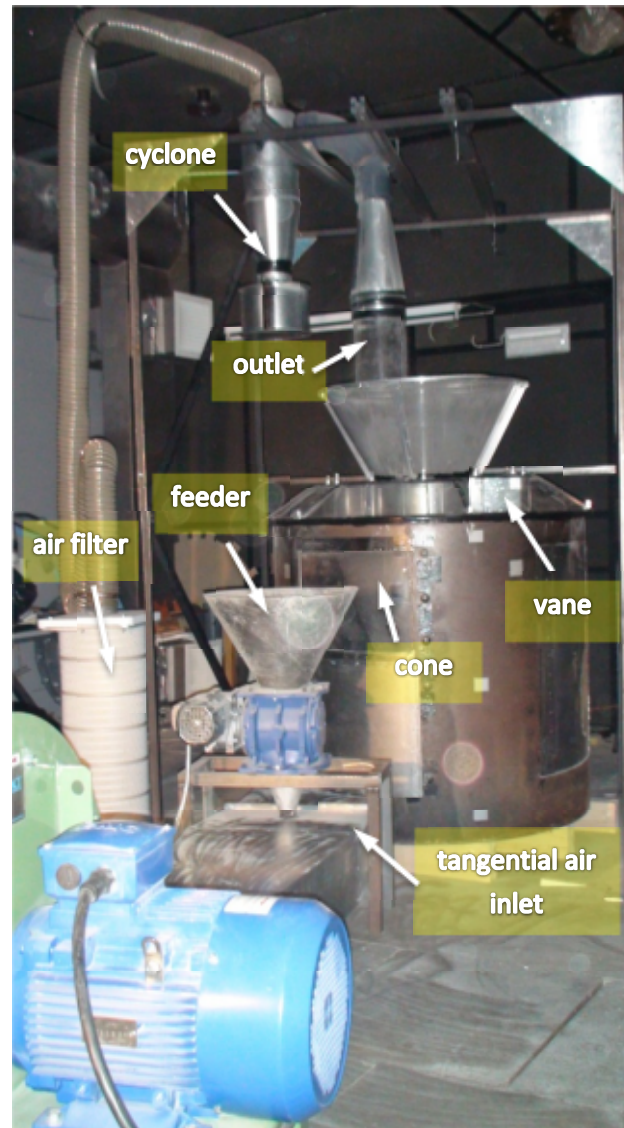
Figure 3.6: The actual built model classifier
