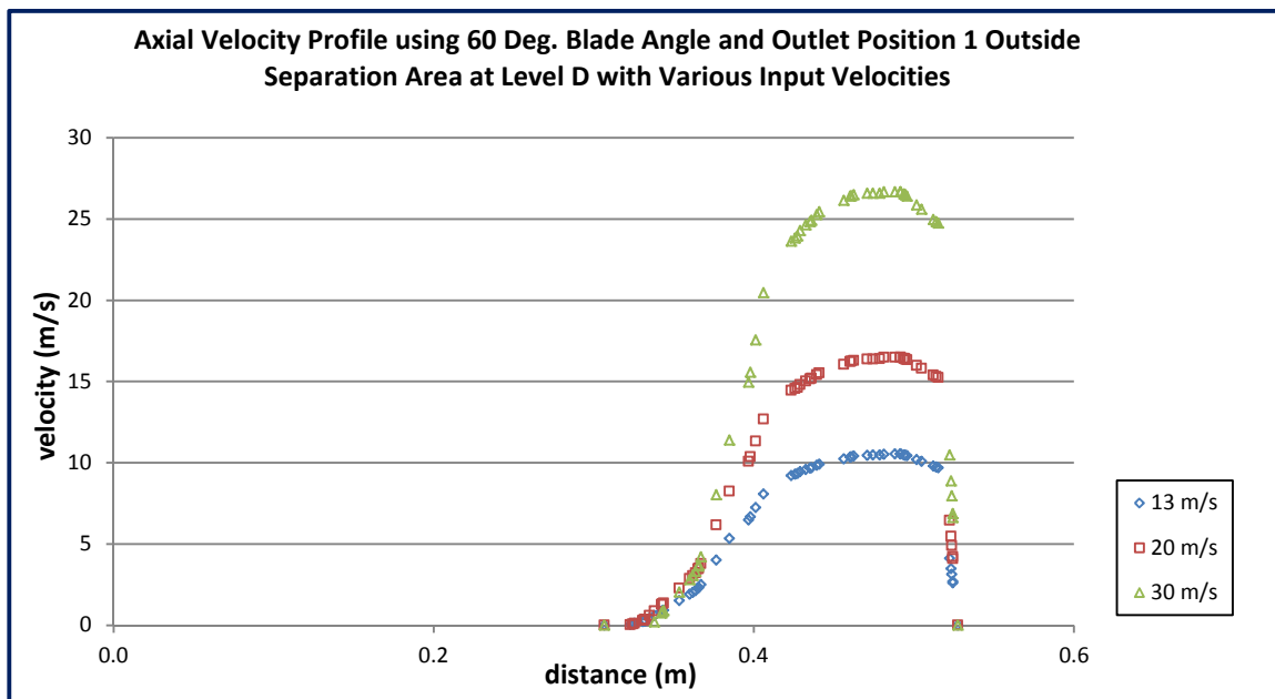
Axial velocity profile outside separation area at Level D for various input velocities (60 degrees vane angle)
