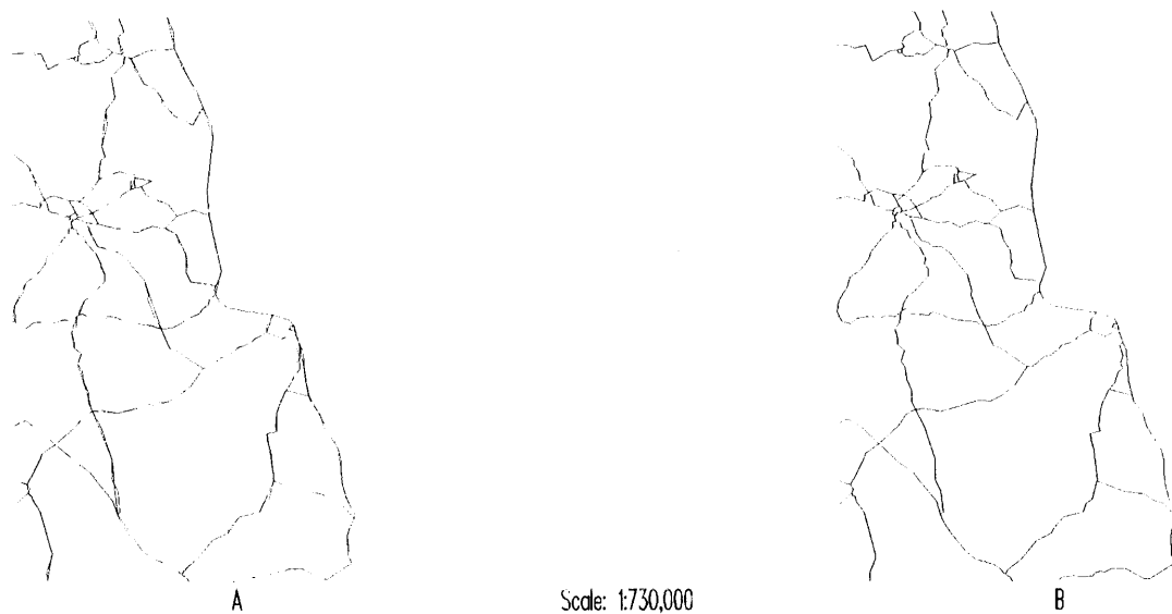
Figure 5.36: In (A) an overlay of original (in Red, 866 point) and digitally simplified map (in Green), 190 points (78.07 per cent data reduction), produced by a tolerance of 280 m (MR1). In (B) an overlay of original (866 points) and, digitally simplified map (in Green), 650 points, produced by a tolerance of 26.070 m (TPF), 24.95 per cent data reduction. Width of drawing line= .15 mm, represents 109.50 m on the ground. (Study Area 3).
