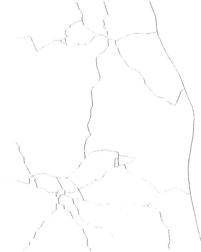
Figure 5.33a: An overlay of two maps at 1:200,000 (Study Area 3). Original map in Red (866 points, 103 arcs). Digitally simplified map (in Green) produced by applying MR1, T = 20.000 m, 688 points, 20.56 per cent data reduction. Due to scale and paper size only half of the map is displayed, Figure 5.33b shows the other half. Width of drawing line = .15 mm, represents 30 m on the ground.
