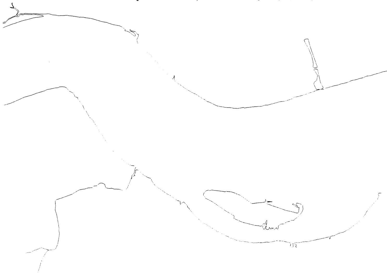
Figure 6.9.2: Due to scale and paper size only half of the map is displayed, see Figure 6.9.1. Simplified map at 1:50,000, 1274 points, 64.25 per cent data reduction from 3563 points database and, 70.30 per cent from 4056 points database. 1) Feature Selection, 2) T_1 = 6.10 m, 3) VD = 33.61 m, 4) T_2 = 2.00 m. Drawing line width: .15 mm, represents 7.5 m on the ground. (Study Area 1).
