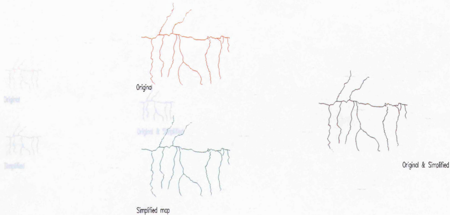
Figure 6.20: Two maps at 1:250,000. Original map in Red (2257 points, 25 arcs), and the simplified map in Green (348 points). 1) Features Selection, 2) T_1 = 32.573 m, 3) VD = 37.248 m, 4) T_2 = 10 m. 84.59 per cent data reduction from 2257 points database, and 97.89 per cent from 8717 points database. Drawing line width: .5mm, represents 37.5m. (Study Area 1 -Drainage Coverage).
