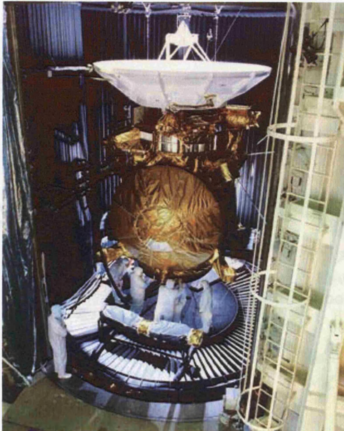
Figure 3.1 The Huygens probe (gold dome) being mounted onto the Cassini spacecraft prior to spacecraft testing and launch. Courtesy NASA/JPL-Caltech.
