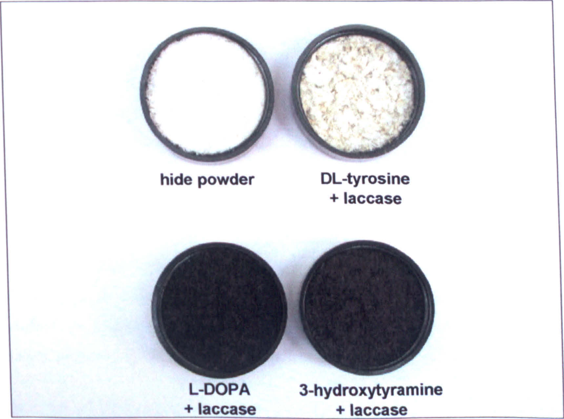
Figure 5.10 Hide powder coloured by aminophenol-laccase treatments
