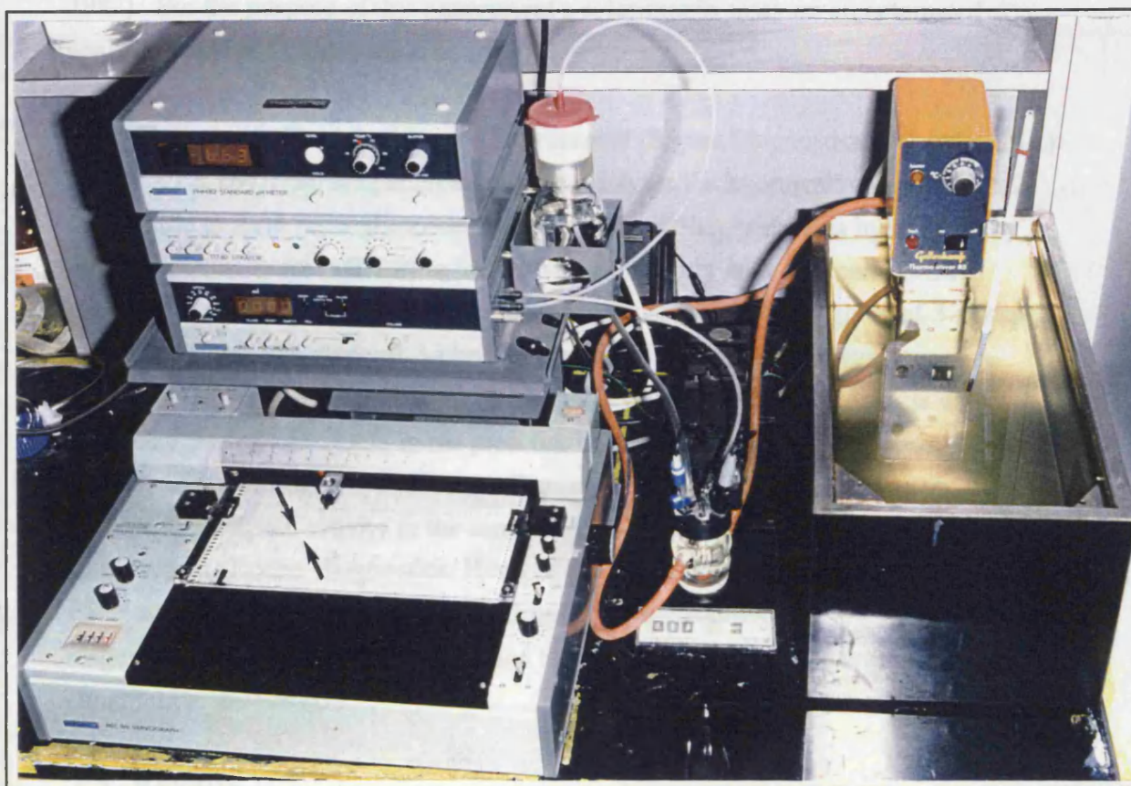
Figure 7.5 Potentiometric titration of fatty acids produced by phospholipase A_2 using a pH stat (see arrows)
