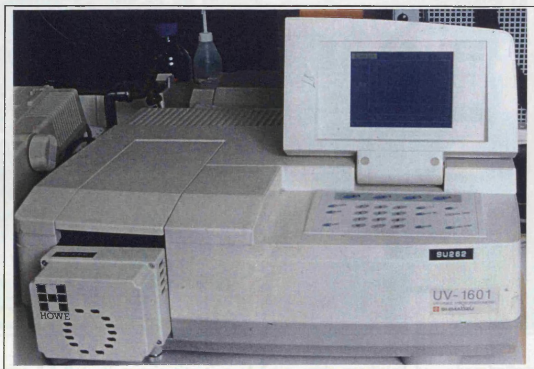
Figure 7.4 UV-spectrophotometer used for carboxypeptidase (A and B) assay
