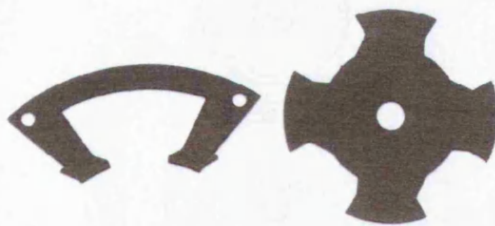
Figure 6.31 :- Actual laminations made by wire erosion method.
