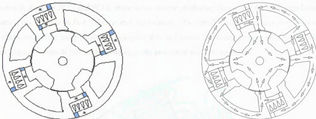
Figure H.13, H.14 :- Magnets flux rotated 90 degrees. Shaded areas to be air or aluminium. More complex steel laminations, shaded areas of air or aluminium to reduce flux leakage paths, risk of saturation in sections other than stator poles (surrounding the magnets) (* in diagram), magnet size is reduced. Very long flux paths.
