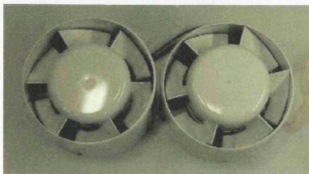
Figure H.37 :- Assembled induction motor (left) and PMFSM (right).
