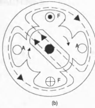
Figure 2.45 :- Inductor Alternator based on a Switched Reluctance lamination [50].
