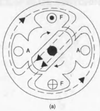
Figure 2.45 :- Inductor Alternator based on a Switched Reluctance lamination [50].
