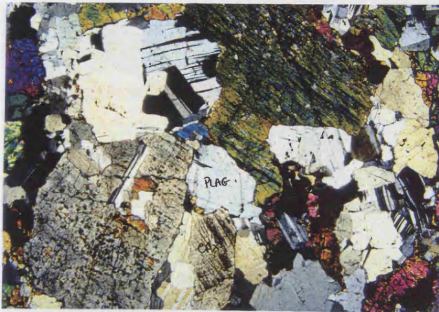
Fig. A.IV.8. XPL view of Fig. A.IV.7. Note the deformation twins in some plagioclase crystals. Field of view 8 mm.
