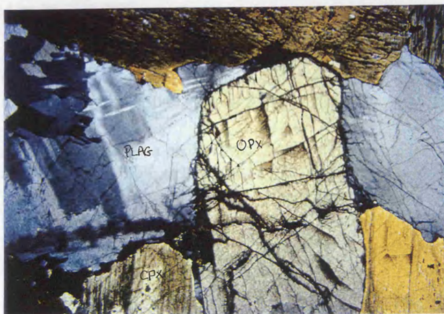
Fig. A.IV.12. XPL view of Fig. A.IV.11. Note the internal deformation in plagioclase and the relatively smoothly curved grain boundaries. Field of view 8 mm.
