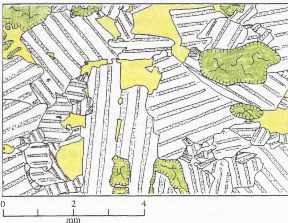
Fig. 3.6 Traced photomicrograph of a portion of a troctolite from 52.98 mbsf. Note the clinopyroxene within plagioclase, elongate parallel to the plagioclase twin orientation (just below the centre of the figure).
