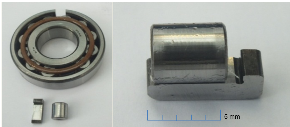
Figure 3-16: The sample of a cylindrical roller bearing for measuring the surface texture.
