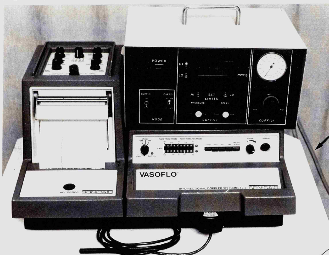
Figure 16. 10MHz Doppler pencil probe linked to a chart recorder. Arrowed on the right is the compressed air pipe which drives the control unit on top of the Vasoflo.
