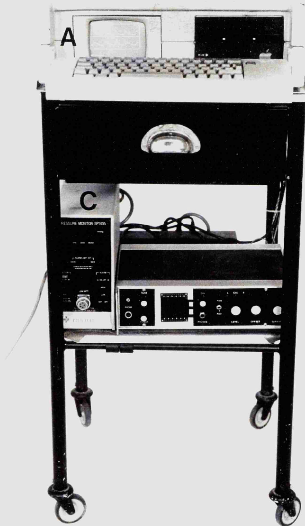
Figure 33. Apple 2E microcomputer (A) linked to a Doppler Flowmeter (B) and a Gould pressure monitor (C).
