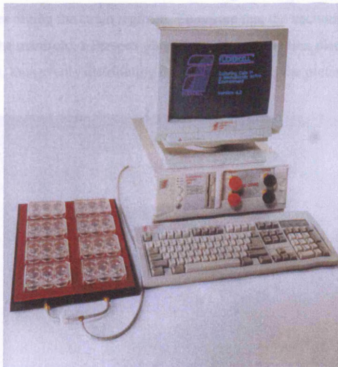
Figure 8- The Flexercell Strain Unit showing the vacuum manifold containing the Flexercell plates.
