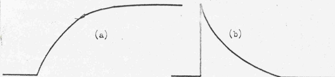
Fig. 4.5 : Effect of deep - trapping for the case \tau < t_t . (a) is the integrated pulse; the rising edge is extremely non - linear. (b) is the current pulse; no discontinuity at t_t appears.
