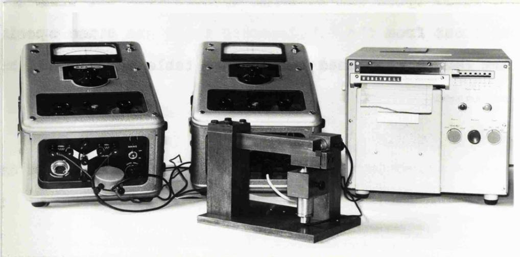
**Fig. 5.4** Photograph showing the dynamometer complete with measuring equipment, consisting of two Pendeford multimeters and a U.V. recorder.
