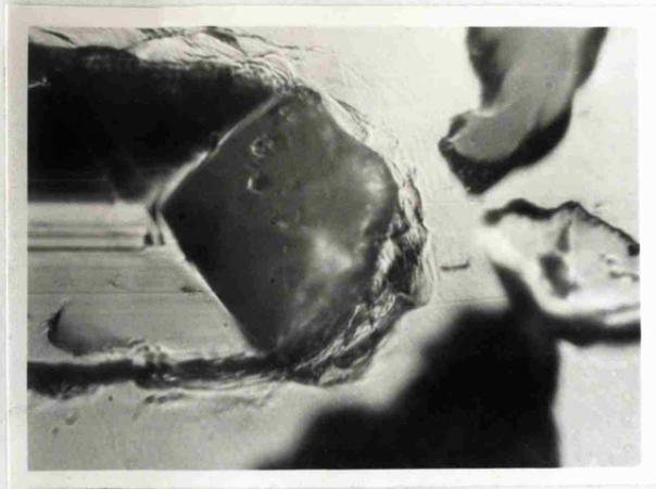
**Fig. 6.6 Vickers indenter facet-first orientation, material B.D.M.S., load 500g, magnification X 440.**
