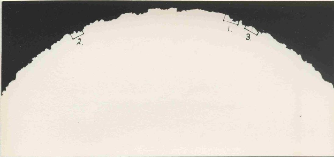
Fig. 7.16 Photograph of diamond dressed 60 grit wheel, X 7.
