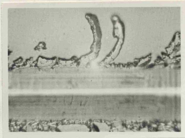
Fig. 6.14 Repeated tracks Vickers indenter facet-edge orientation, material hardened 1% C steel, load 500g, magnification X 440.
