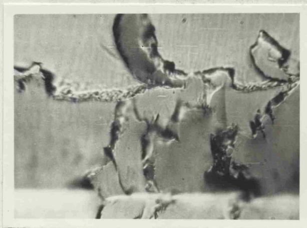
Fig. 6.15 End of repeated tracks Vickers indenter facet-edge orientation, material hardened 1% C steel, load 500g, magnification X 1045.
