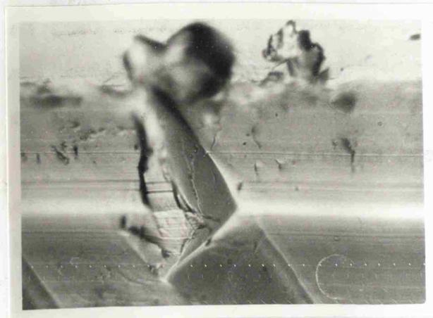
Fig. 6.11 Repeated track Vickers indenter facet-first orientation, material B.D.M.S., load 500g, magnification X 440.
