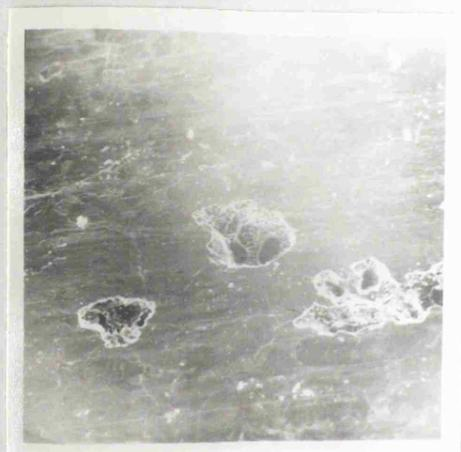
Fig. 7.33 Glazed abrasive pin viewed at  $45^\circ$ , X 70
