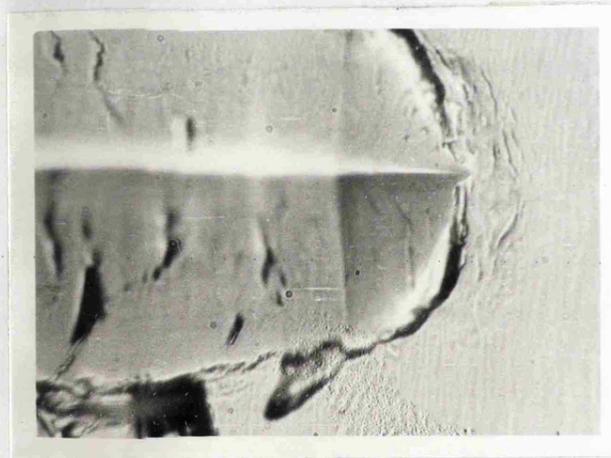
**Fig. 6.7 Vickers indenter facet-edge orientation, material hardened 1% C steel, load 500g, magnification X 1045.**
