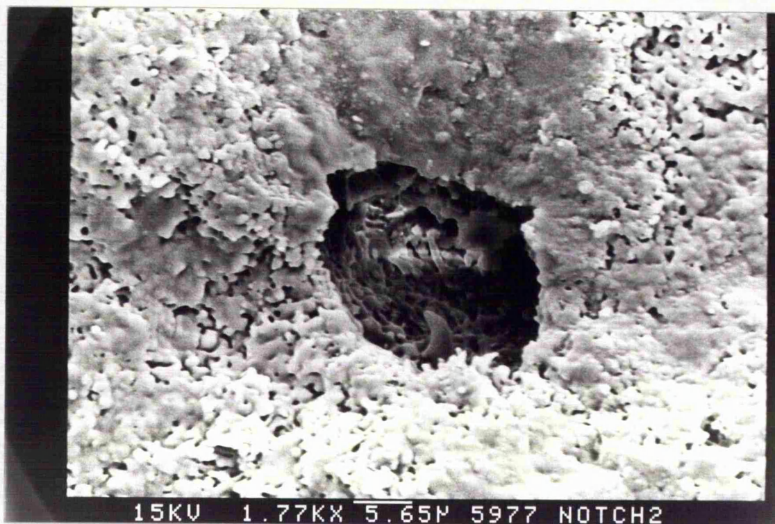
Plate 5.1b. A close-up of the pre-existing cavity in the same specimen at 1770x magnification. Note the partially crystalline partially amorphous structure.
