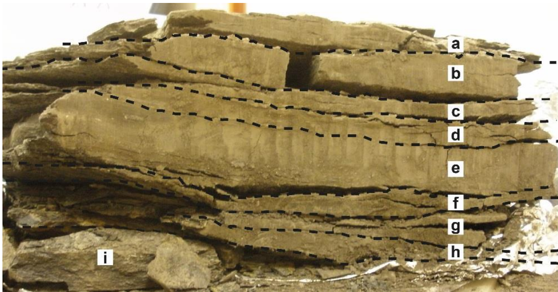
Figure C.1: Coldstream block for detailed study, vertical section, from 33-40 cm on log. Letters indicate described beds. Block is about 30 cm across.
