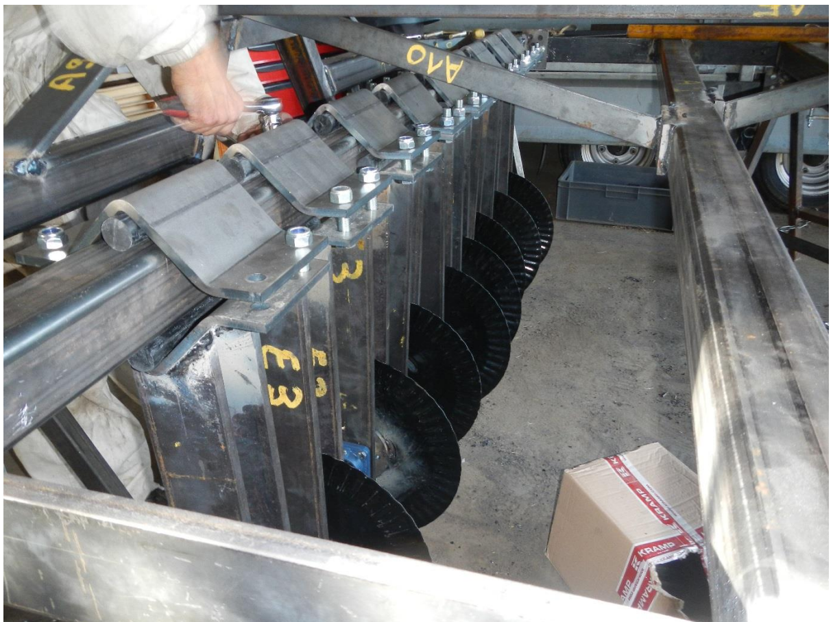
Figure 7: some metal components are too solid to be practically bent in the required shape using basic equipment.
