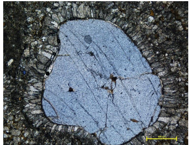
Plate 5.4 Tmessah Member. A-TM12, rounded quartz clasts with reddened rim cements (x5, ppl). B-TM15-very coarse spar cement infilling pore spaces between quartz clasts (x5, cpl). C-TM21, bimodal sorting of clasts. Large clasts have surface fracturing, meniscus cements which are locally reddened (x5, cpl). D-TM24, rim cement of bladed spar crystals (x5, cpl). E-TM24, secondary mosaic spar infilling rootlet (x5, cpl). Scale bar is 500μm in all microphotographs.
