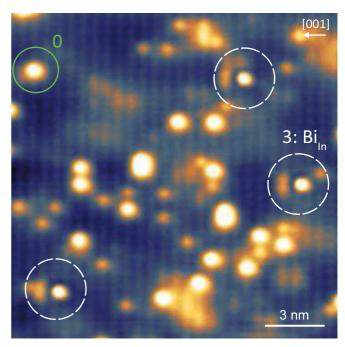
FIG. 7. High-resolution filled state X-STM image with potential Bi<sub>In</sub> antisites [class (3)] with a valence of 5 in the surface layer next to commonly observed isovalent Bi<sub>P</sub> substitutional atoms. An isovalent Bi<sub>P</sub> atom in the cleavage plane [class (0)] is marked for comparison. The image is taken on F2 in sample B at  $I_T = 40$  pA and  $V_{\text{bias}} = -2.5$  V. The growth direction is indicated by an arrow.
