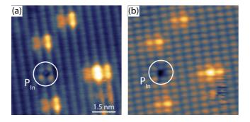
FIG. 6. High-resolution filled (a) and empty (b) states X-STM images of a P<sub>In</sub> antisite in the surface, which is marked with a white circle. The images are acquired from the same spot of QW 2 in sample B at  $V_{\text{bias}} = -1.9$  V and  $V_{\text{bias}} = 1.5$  V with the same  $I_T = 30$  pA. The color ranges in both images are adjusted independently.
