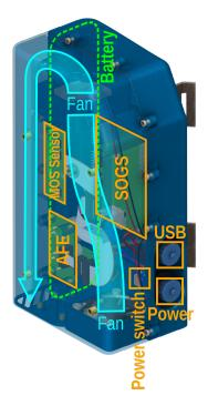
**Figure 6.** Cutaway of the prototype Zephyr enclosure, showing the layout of vital components and interfaces. Major components are labelled in orange, including an Alphasense AFE electrochemical sensor, which is not the subject of this paper. The MOS instrument boards are suspended away from the casing wall to allow air to flow past both sides.
