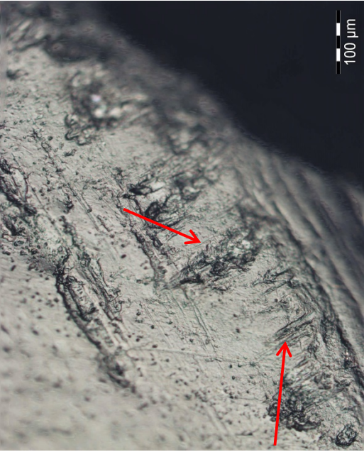
Figure 6-22: FEK 016, Point 12 x200 EFi; short transverse striae running back from edge indicated by red arrows
