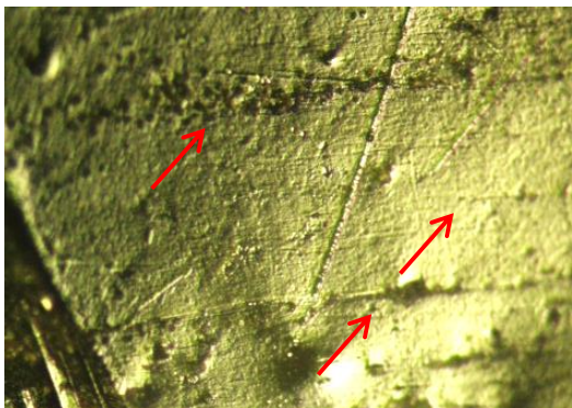
Figure 6-97: FRL 428, Point 5 x100; transverse striae indicated by red arrows
