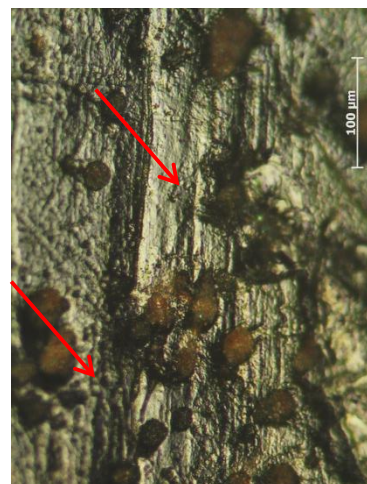
Figure 7-4: FDM 002, Point 5 x200; axial striae indicated by red arrows
