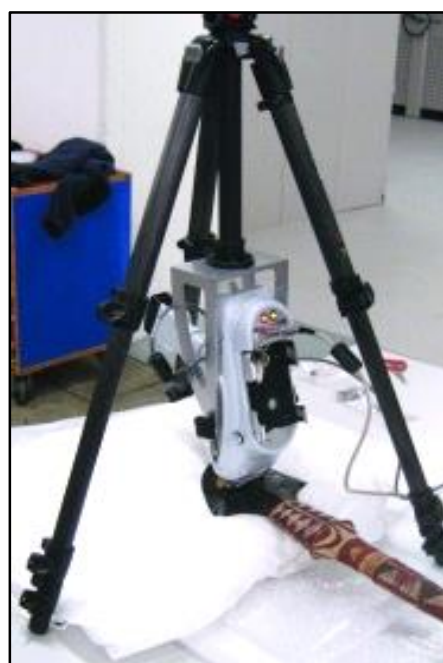
Figure 5-22: Bruker-Tracer III-V PXRF machine being used for non-destructive testing of a hafted obsidian blade (Torrence et al. , 2013: 295)
