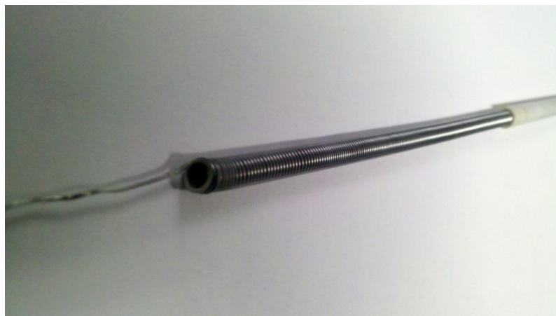
Figure 3.27 Showing a coiled tantalum heating element wire
