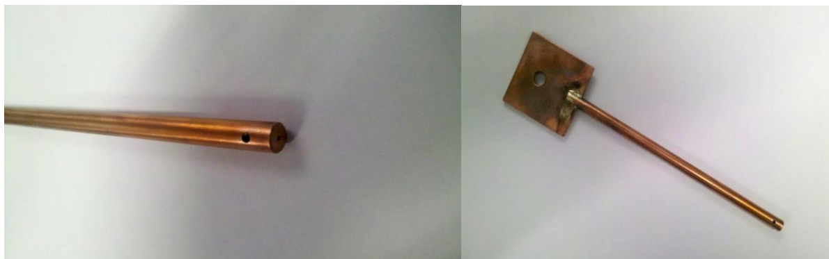
Figure 3.23 A design of copper connector; Left is a hole to place heating element wire and fix with grub screw, Right is the connecting plate which will hold connector of a high current power supply.
