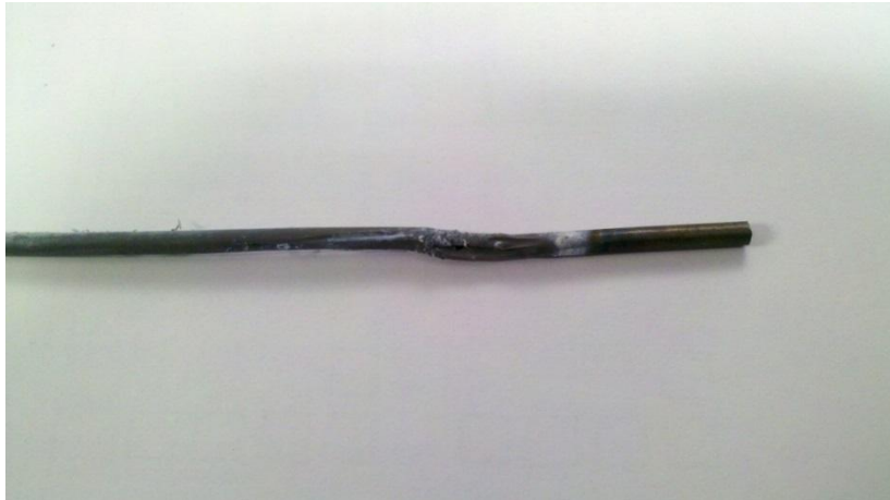
Figure 3.26 Kanthal A1 wire showing oxidation and split of the wire due to 'blow out'
