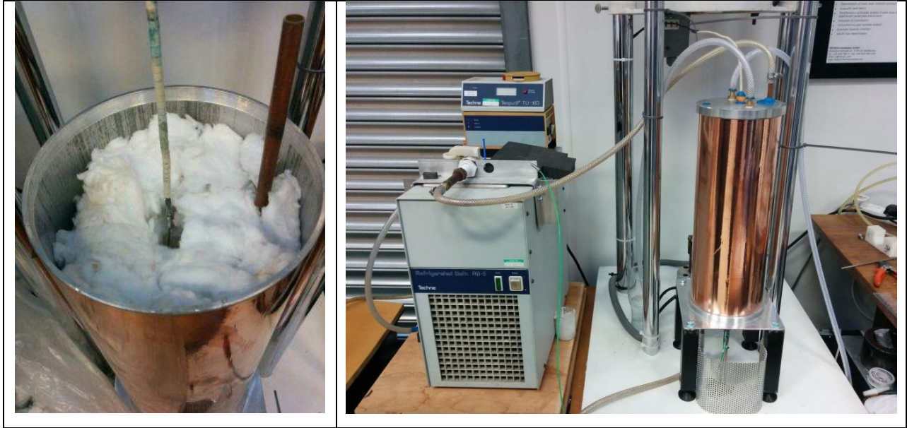
Figure 3.34 The left shows the radial heat furnace filled with insulation, superwool, and the right shows the full set up of the experiment with the refrigeration bath
