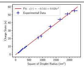
FIG. 3. Plot of the droplet charge state versus the square of the minimum droplet radius needed to form that particular charge state. The red curve is a fit to the experimental data. The horizontal error bars originate from the statistical uncertainties in determining the sizes of the droplets and the vertical bars from the uncertainties in the appearance of specific charge numbers amongst the series of higher charge states.
