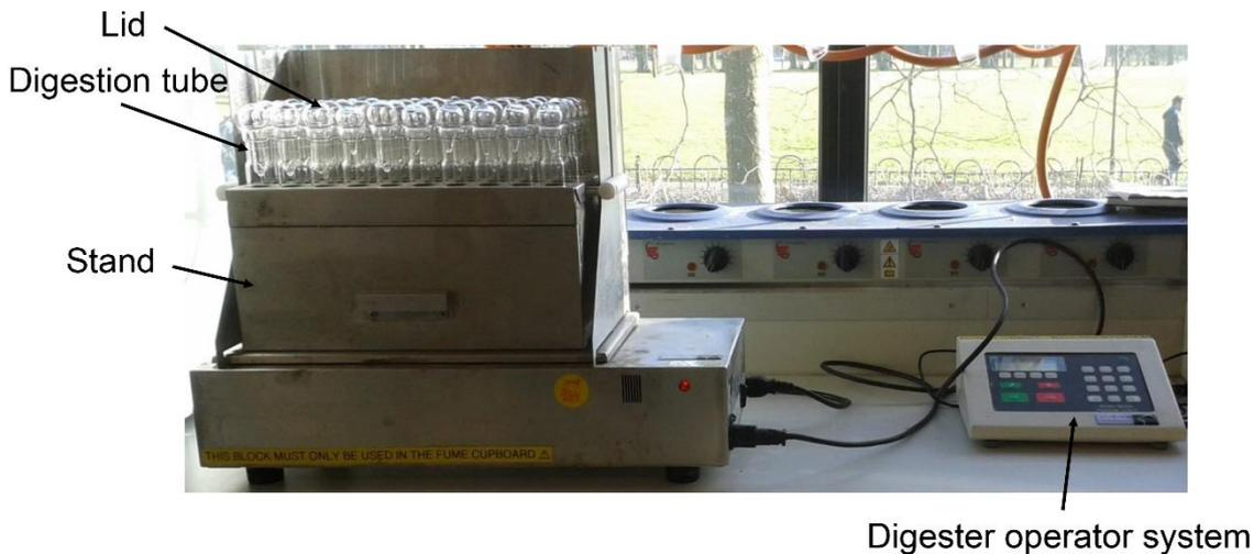
**Figure 3.1: Digestion Unit structure.**
