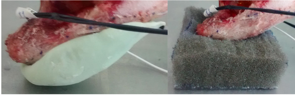
Figure 5.2: Two greater trochanter protectors. Left: PMMA, right: foam.
