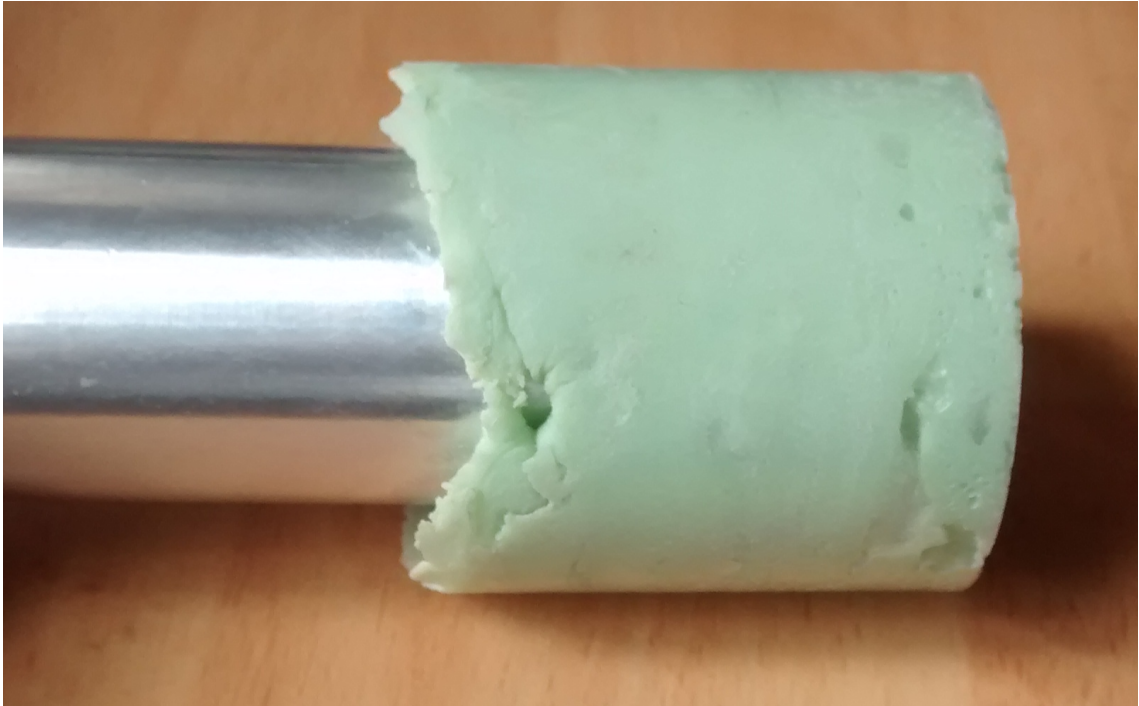
Figure 3.3: The result of the first PMMA test, outer cylinder removed. The void spanning the entire thickness of the side of the cement is visible in the centre of the image.
