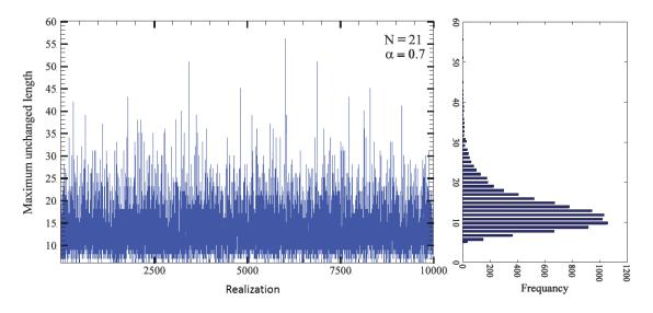
**Figure 2.** The maximum time interval during which a network resists against any change (long-lived states). The left panel depicts this time interval for networks with 21 nodes in various paths (10,000 realizations). The right panel illustrates that the maximum time intervals follow a Poisson distribution.
