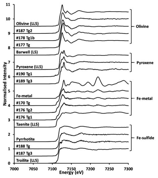
Fig. 6. The Fe-K XAS of other terminal grains in the Stardust keystones studied, including olivines, pyroxenes, Fe-metals, and Fe-sulfides, compared to standard reference materials and chondritic materials, Barwell (L5) and Tuxtuac (LL5).
