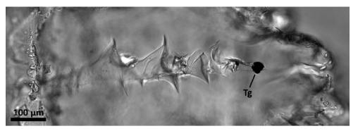
Fig. 3. A keystone with a NWA 10256 CR2 chondrite magnetite terminal grain, shot into aerogel at 6.10 km s<sup>-1</sup> using the lightgas gun at the University of Kent (Burchell et al. 2008). The remaining track stylus cut from the aerogel, minus the bulbous region, measures 650  $\mu$ m with a ~30  $\mu$ m terminal grain.
