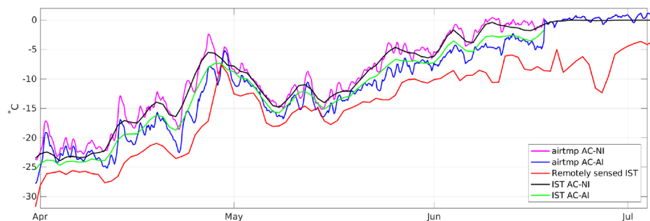
Figure 4. Time series of atmospheric forcing temperatures before the corrections (experiment AC-NI, magenta) and after the correction (experiment AC-AI, blue). Also shown are IST from the reference experiment AC-NI (black line), the experiment with corrected forcing (green) and the observed IST based on remote sensing observations (red line). All time series are from a position at 87.1°N and 184.5°W. The atmospheric forcing is plotted every third hour; both the modeled and remotely sensed IST are plotted as 72 h averages.
