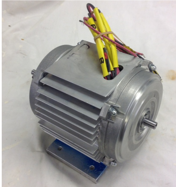
Figure A.3: The frame of the prototype motor.
