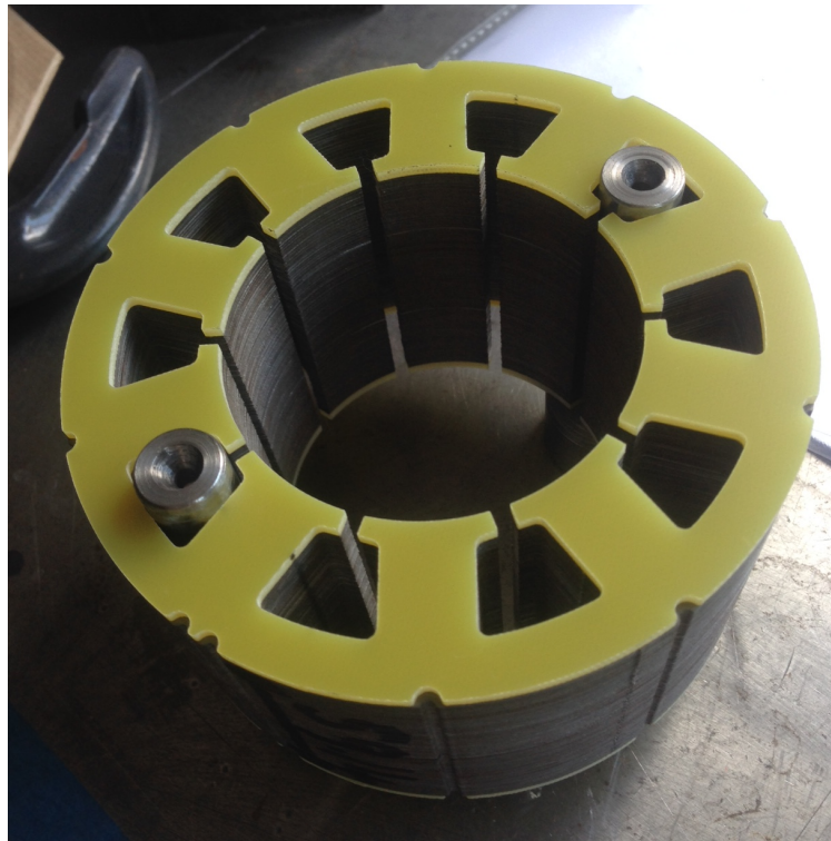
Figure A.2: Prototype machine stator core.
