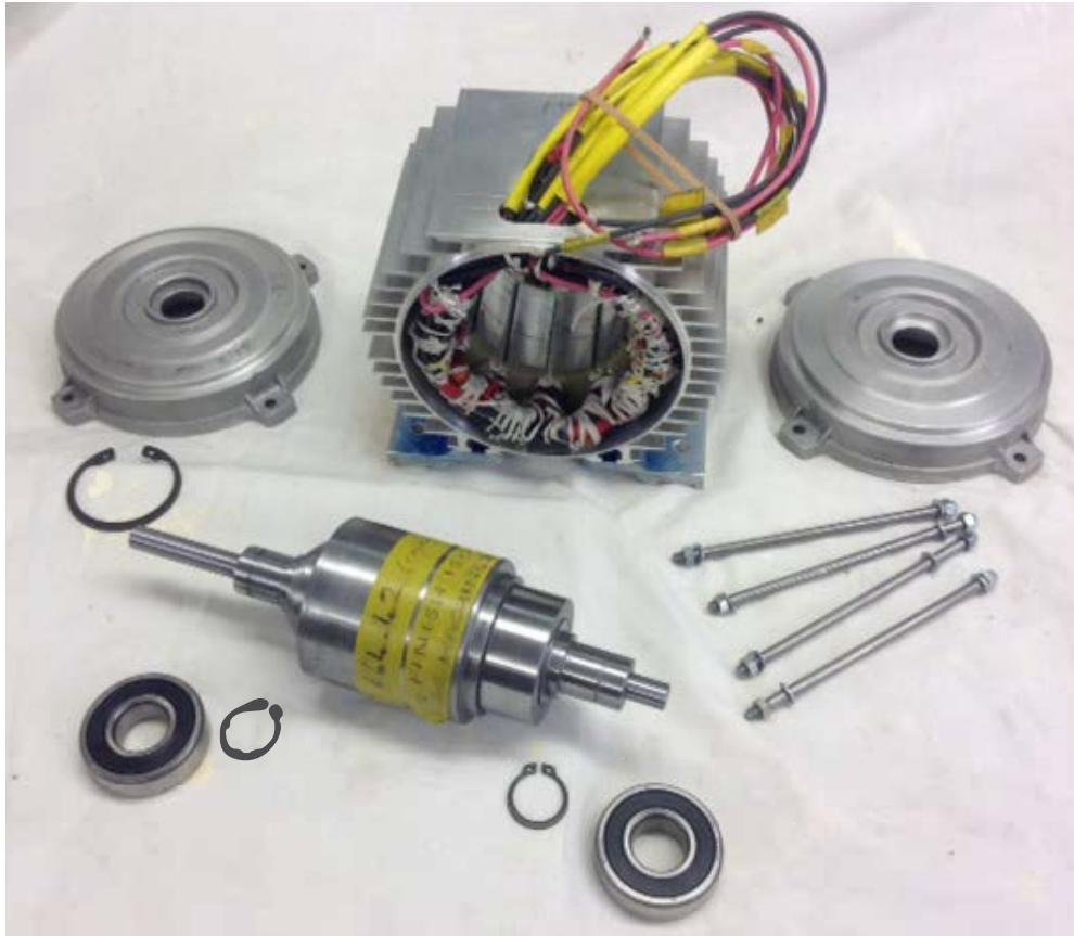
Figure A.1: Stator, rotor, covers and bearings of the prototype motor.
