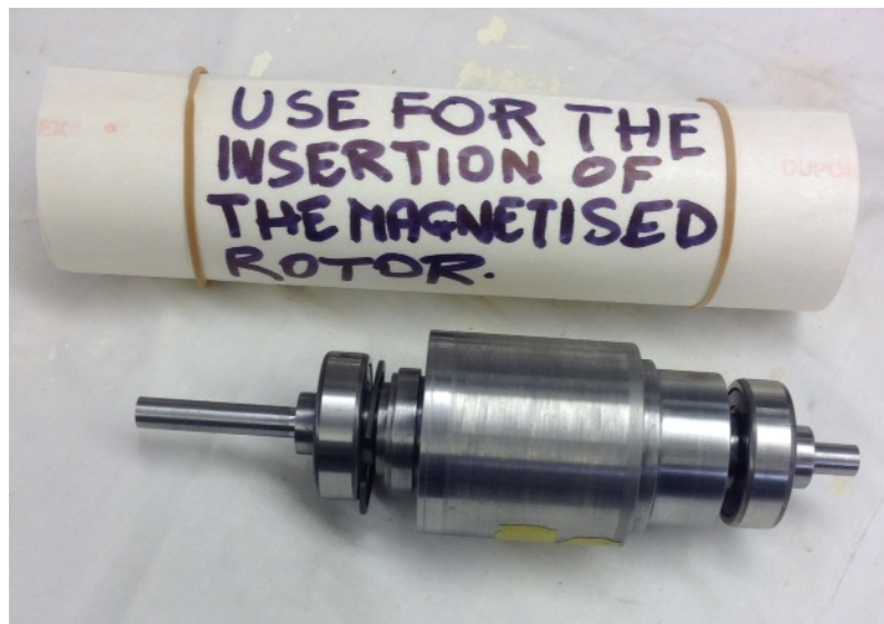
Figure A.4: The cylindrical shaped rotor, including bearings.
