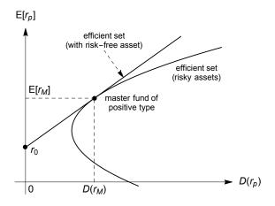
FIG. 3. Efficient sets (frontiers) for portfolio problem (45): expected rate of return versus deviation of optimal mean-deviation portfolios when the risk-free asset is available (security market line for  $\mathcal{D} = \sigma$ ) and when it is not.
