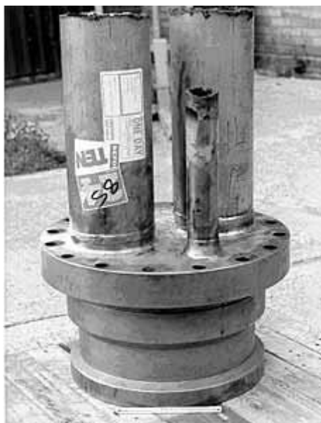
Figure 1-1 Hydrogen assisted failure of SDSS hub and two pipes, removal from the manifold [13]
