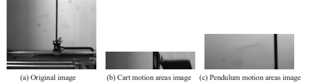
Fig. A.1. Find the motion areas of cart and pendulum from the original image.
