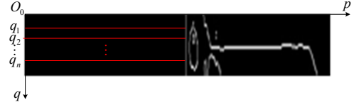
Fig. A.4. Cart position is determined using the line scan algorithm.
