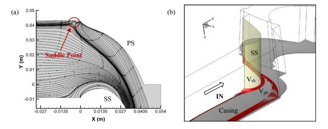
Fig. 3 (a) Flow visualization over the stator 1 axisymmetric casing showing the separation of oncoming casing boundary layer (saddle point) by the streamlines (b) The same surface showing by the ribbons the pressure side horseshoe vortex interacting with its suction side branch.
