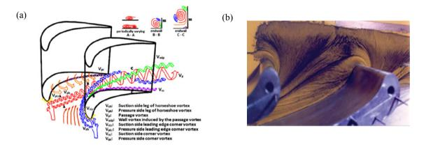
Fig. 1: (a) Secondary flows through a turbine blade passage [4], (b) visualisation of the horseshow vortex [7].
