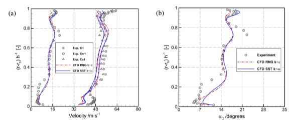
Fig. 2. Radial distributions of pitch mass-averaged (a) absolute (C1), axial (Ca1), and tangential (Cw1) velocity components and (b) yaw angle at 8.8 mm downstream of the rotor exit plane.
