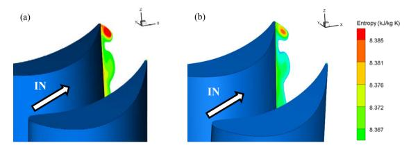
Fig. 7. Entropy distributions at the rotor exit off-design: (a) axisymmetric casing, (b) contoured casing of new design.
