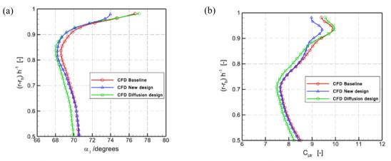
Fig. 5. Radial distributions of predicted pitch-averaged (a) yaw angle 8.8 mm downstream of the upstream stator exit plane and (b) total pressure loss coefficient 8.8 mm downstream of the rotor exit plane.
