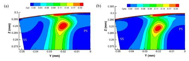
Fig. 6. Contours of total pressure loss coefficient at 8.8 mm behind the upstream stator off design: (a) axisymmetric casing, (b) contoured casing by the new design.
