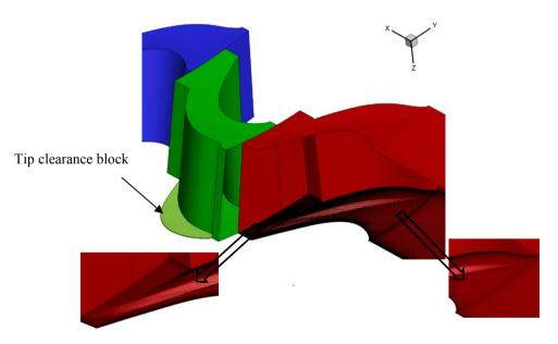
Fig. 4. Non-asymmetric casing NURBS imported in ICEM CFD.
