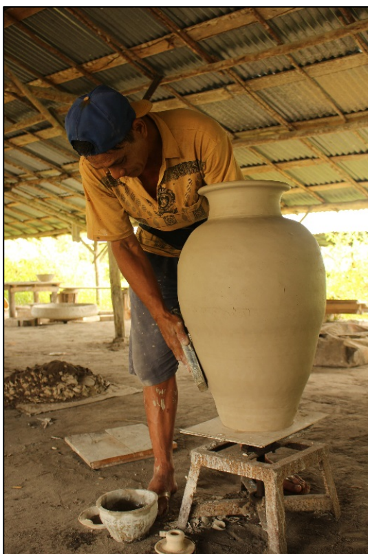
Figure 3.20 - Potter joining two, wheel-thrown jar halves together by hand at the Tajau Mas Pottery, Singkawang, Kalimantan, Indonesia, 2013. Image by BN.
