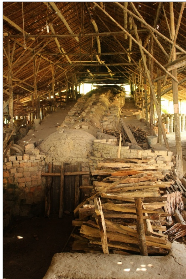
Figure 3.25 - Wood-fired, traditional dragon kiln still being used by the Tajau Mas Pottery, Singkawang, Kalimantan, Indonesia 2013. Image by BN.
