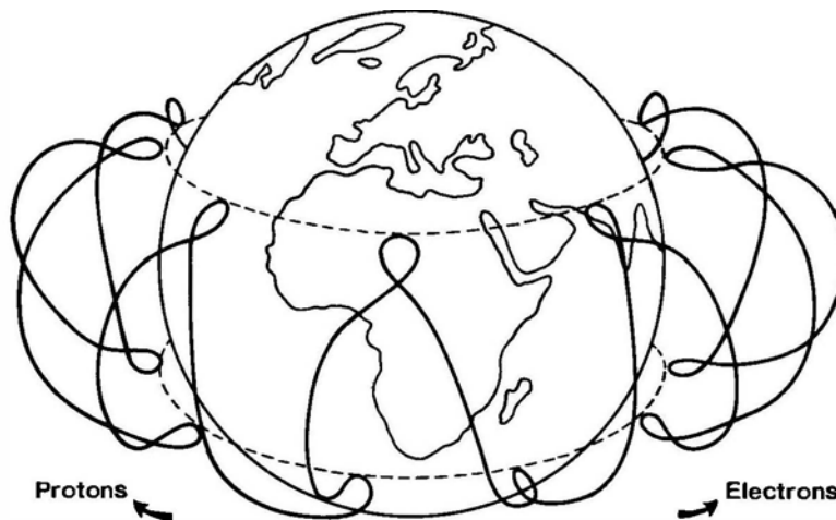
Figure 1.3 Illustration of the direction of energetic charged particles drift in the earth's dipolar magnetic field; electrons drift eastward in the direction of the earth's rotation, and protons drift westward. Taken from Kivelson and Russell (1995).
