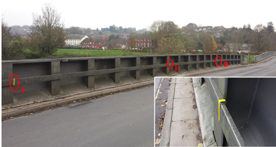
Fig. 9, IMUs deployed at sensor locations F, E & D (see Fig. 7), insert shows how IMUs were simply taped to the horizontal member adjacent to the vertical web stiffener.
