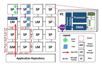
Fig. 1: 4x4 platform instance, partitioned into 2x2 clusters.
