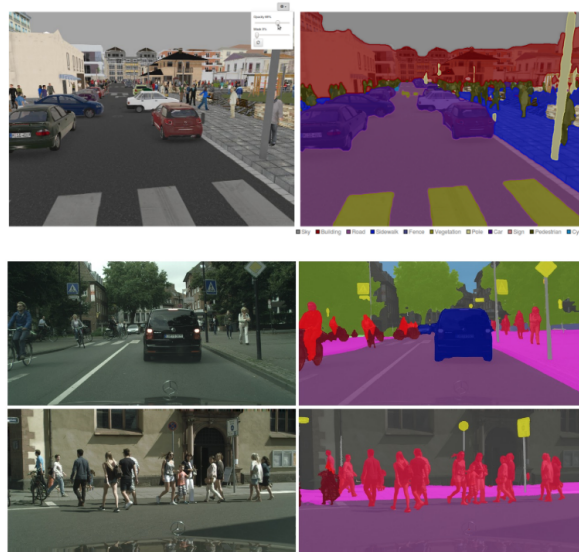
Figure 12. An example of envelope extraction from different images as input. Top: image from devblogs.nvidia.com/image-segmentation-using-digits-5/ ; bottom: image from http://vladlen.info/ .
