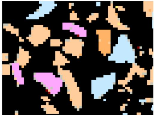
*Figure 5.4: a. Section of the overall coloured chalcopyrite mineral map. b. back scattered electron image from a small section. c. Corresponding mineral map image to the back scattered electron image. (beige = chalcopyrite)*
