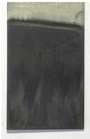
*Figure 3.7: Photograph of the Ni cathode surface after electrolysis of PbS in Ethaline for 5 hours at a constant 1.5 V.*
