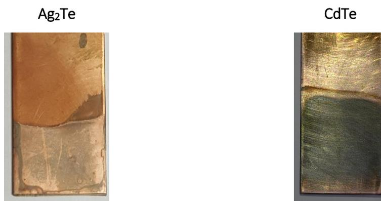
*Figure 4.17: Shows the resultant cathodes (Cu left, Ni right) of the recovery experiments conducted on the transition metal chalcogenides for 24 hours at a constant 1.5 V in Ethaline.*
