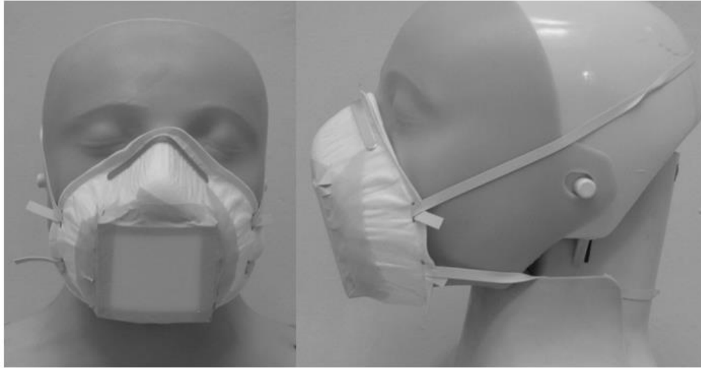
Figure 1.5 FFP30 masks incorporated with gelatine filters used in Williams et al. (2014) This was reproduced from Williams et al. , 2014 (open-access article permitting unrestricted use).
