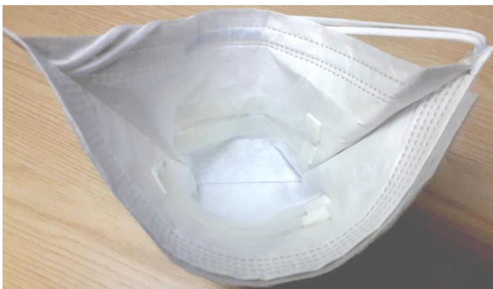
Figure 4.3 Duckbill mask integrated with four 3D printed 9x1cm PVA strips
