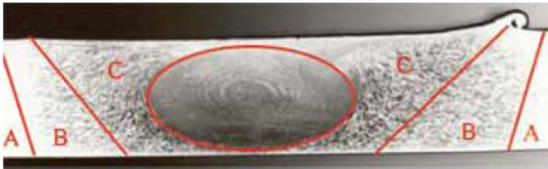
Figure 2-11. Microstructural zone classification in a friction stir weld in Al 2024 alloy (A: Parent material, unaffected by process; B: HAZ, thermally affected but with no visible plastic deformation; C: TMAZ, affected by heat and plastic deformation) [57].
