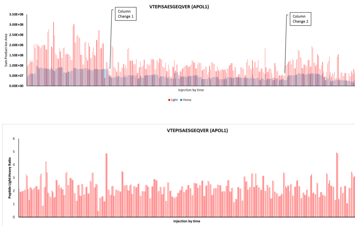
Figure 4-10: Systematic change in absolute ion intensities due to chromatographic column changes did not affect light:heavy ratio measurements
