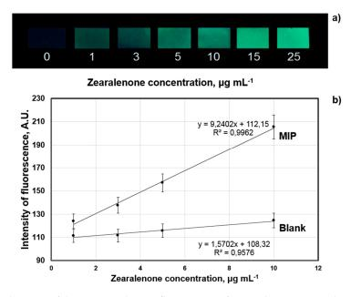
**Figure 8.** Digital images of the MIP membranes fluorescence after incubation in zearalenone-containing  $(1-25 \ \mu g \ mL^{-1})$  aqueous samples (a). Typical calibration plot of the MIP-membrane-based smartphone sensor system for zearalenone detection: smartphone sensor response generated by MIP and blank polymeric membranes as a function of zearalenone concentration registered by Spotxel<sup>®</sup> Reader smartphone application (Sicasys Software GmbH, Heidelberg, Germany) (b).
