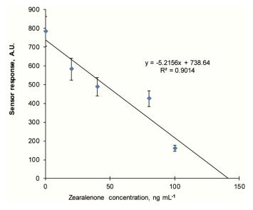
**Figure 9.** Typical calibration plot of the fluorescent sensor for zearalenone detection in competitive mode using 2-[(pyrene-l-carbonyl)amino]ethyl 2,4-dihydroxybenzoate (PARA) as a fluorescent tracer. Fluorescence of the MIP membranes after incubation in 40 ng mL<sup>-1</sup> PARA solution containing 10–200 ng mL<sup>-1</sup> zearalenone and 10% acetonitrile (working solution for the measurements is 20 mM Na-phosphate buffer, pH 6.0, containing 150 mM NaCl).
