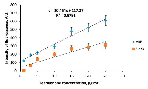
**Figure 6.** Calibration graphs of zearalenone-selective fluorescent sensor based on CDHB-imprinted (MIP) and reference (blank) 1-allylpiperazine-containing membranes (working solution 20 mM Na-phosphate buffer, pH 6.0, containing 150 mM NaCl, 10% acetonitrile and 1–25  $\mu$ g mL<sup>-1</sup> zearalenone). Differential sensor response is a residual between sensor signals obtained by fluorescent sensors based on MIP and corresponding reference polymeric membranes.
